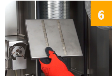
CLEANING THE METAL FILTER BIMONTHLY
